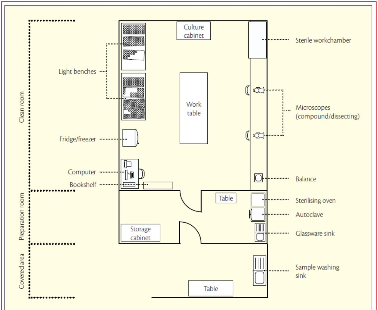
Figure: Typical floor plan and the layout of general plant quarantine/protection diagnostic laboratory [some modification can be made with floor availability and type of laboratory and others]
